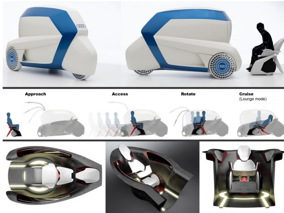
Figure 9. Vehicle's exterior and interior design, with integration of personal mobility device.
