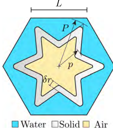
Figure 7: Schematic of the unit cell comprising a hollow N-pointed star.
