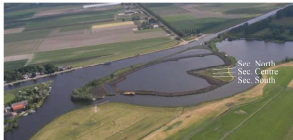
Figure 1. Plane view of the test area at the Leendert de Boerspolder before the start of the failure test ( https://www.stabialert.nl/nl/projecten/ldeb-polder/ ).
