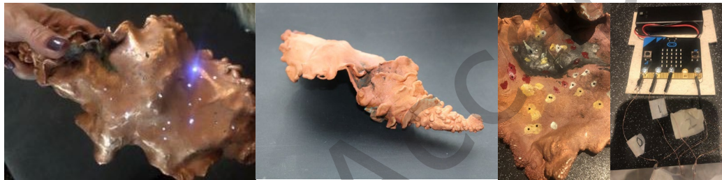
Figure 10. Time capsule is a hand-held piece of digital jewellery that connects a mother with her three daughters. Each daughter is represented by their star constellation. The light constellations light up independently when the wearer tilts the piece in her hand in three different positions, one for each child (a). The piece is made of electroformed fimo and electronics (micro:bit, fairy lights and a battery). (b) The final piece after electroforming process (c) the piece upside-down shows the drills with the marking of the constellations, and (d) the making of the circuit.
