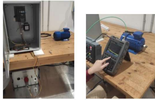
Fig. 2. Experimental set-up: left – LISN, VFD, IM; right – digital oscilloscope, spectral analyzer and IM
