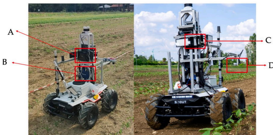
Fig. 2. Component of the main configuration employed during the trial: (A) router, (B) Smart switches, (C) on-board PC, (D) Intel® RealSense™ D435.
