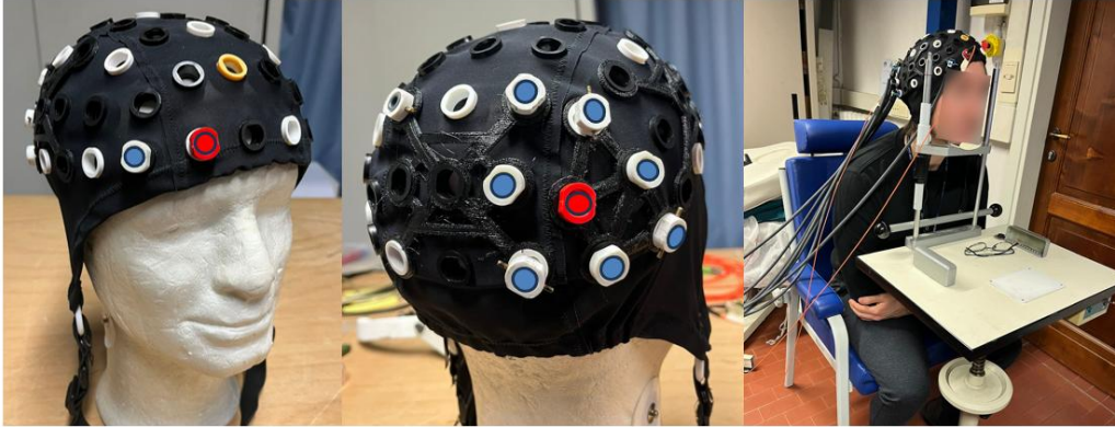
Fig. 2. Picture of the probes geometry where in red are labelled the sources and in blue the detectors.
