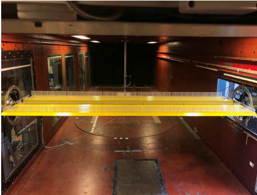
Fig. 15 Section model mounted in the forced vibration rig in the wind tunnel at NTNU, Trondheim, Norway
