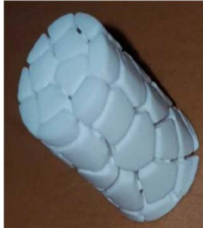
FIG. 3: Pre-fragmented alumina pellet printed by stereo-lithography.
