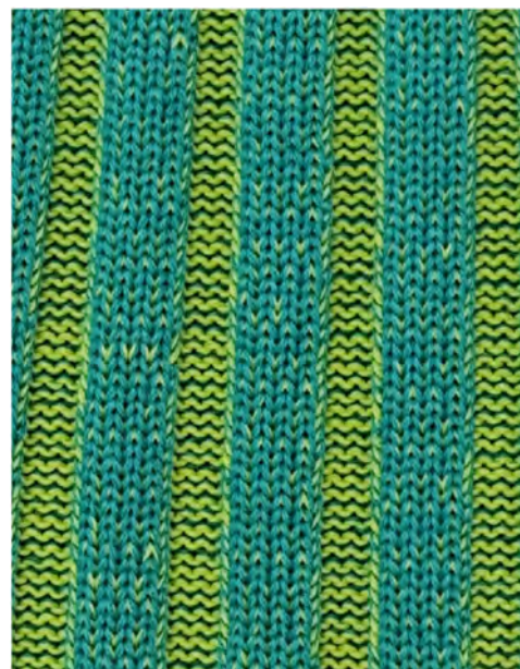
FIGURE 15 Detail of the vertical striped pattern created by the plating technique when applied to a rib knit structure.
