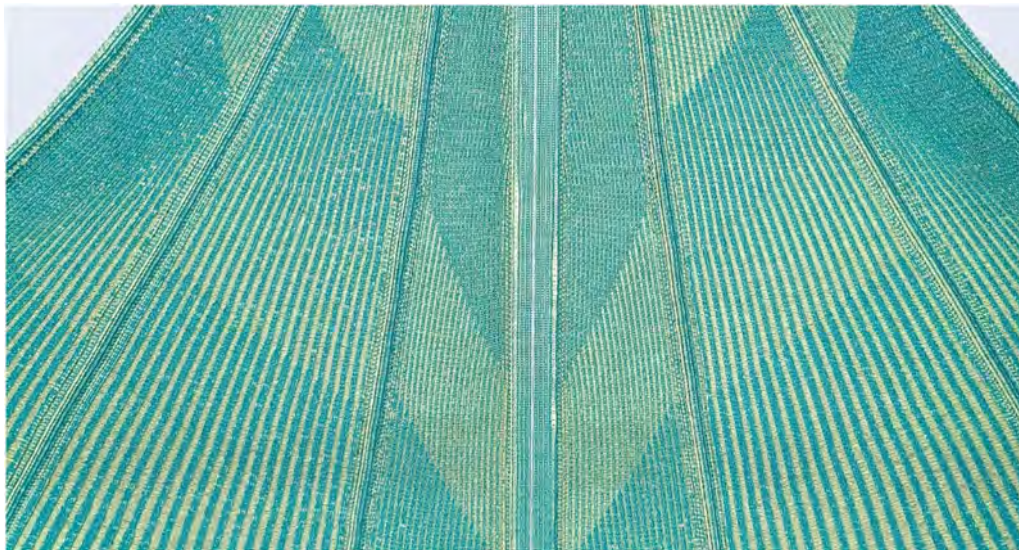
FIGURE 13 Detail of the tubular channels in between the rib portions of fabric.
