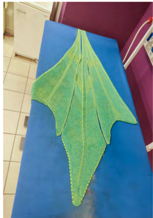
FIGURE 21 Work in progress picture of the three panels before the assembly through linking.
