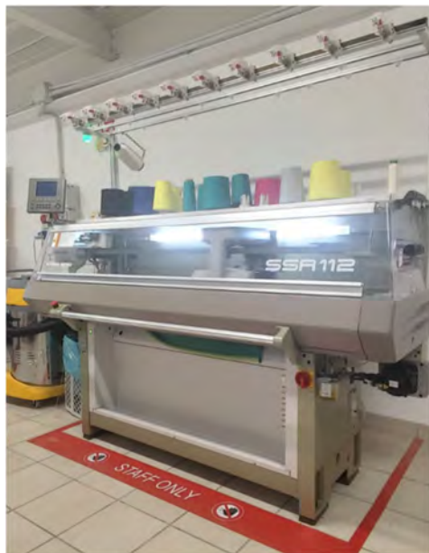
FIGURE 20 The Shima Seiki SSR112 knitting machine used to prototype the Manta.
