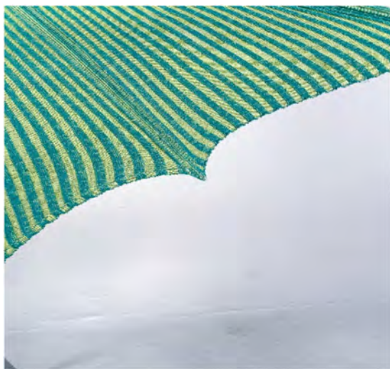
FIGURE 14 Detail of one of the tubular channels hosting the glass-fiber rods in the maximum tensioned state.
