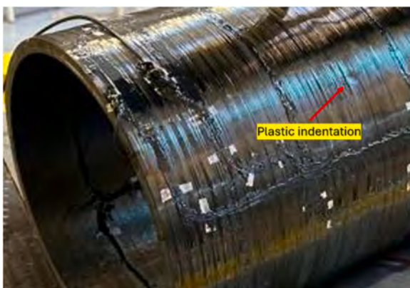
Fig. 17. Magnification of the local plastic indentation visible on the sample after the LVI test.
