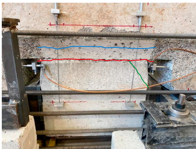
Fig. 3. Damage of the specimen after test.
