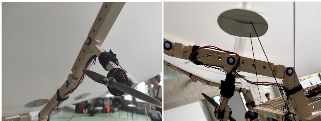
Fig. 7 Detail view of the propeller and of the gondola patches. Left: motor, propeller, and attachment points on the frame. Right: gondola patch with attachment cable.
