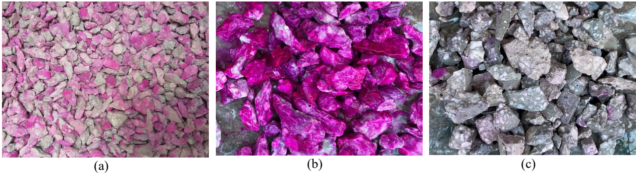
Figure 1– Phenolphthalein test on a bunch of RCA (a) and a pile of alkaline (b) and naturally carbonated (c) RCA
