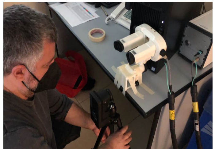
Fig. 3. Setup for the illuminance measurements.
