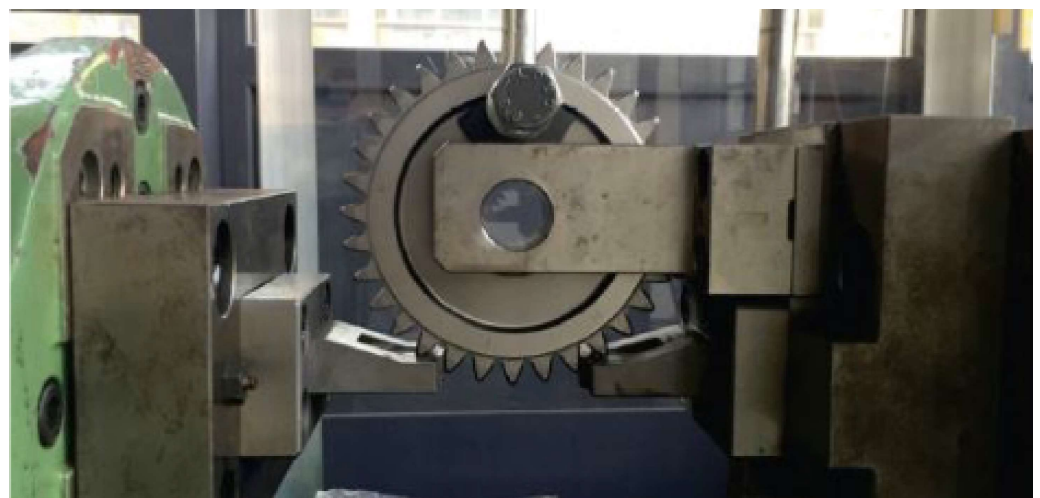
Figure 4. Detail of gear and anvils.
