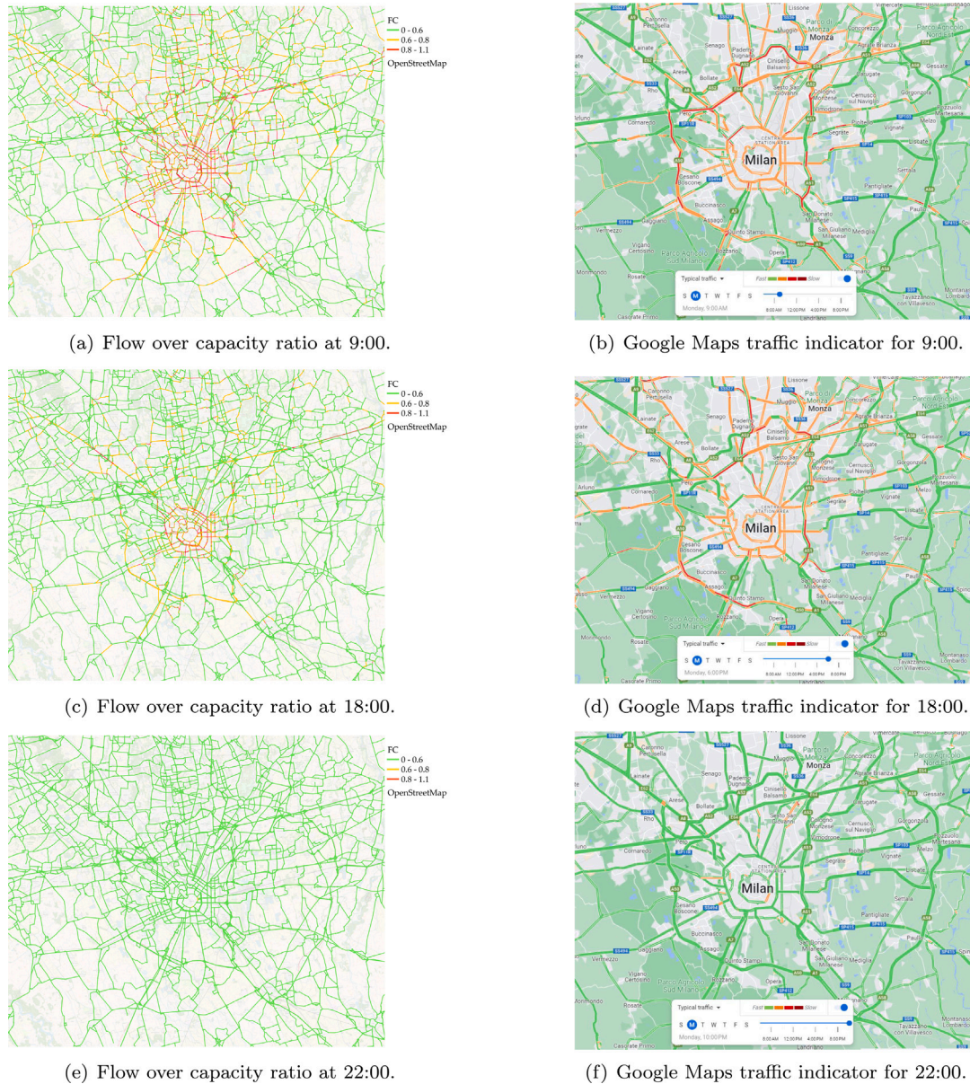
Fig. 9. Comparison of results from traffic model with Google Maps at different times of day. (For interpretation of the references to color in this figure legend, the reader is referred to the web version of this article.)
