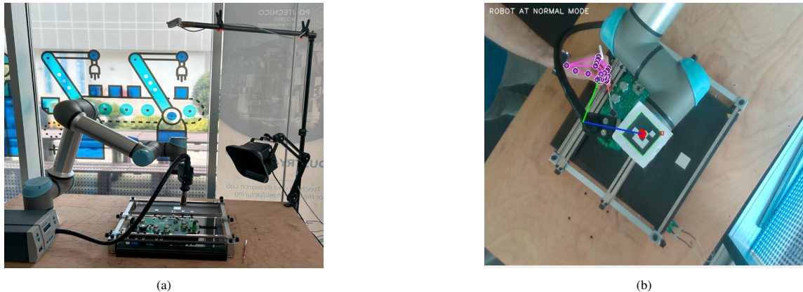
Fig. 2: (a) Experimental setup, (b) localisation of marker (red dot), heater (blue line), hand knuckles (magenta) and minimum distance between hand and tool (green line).
