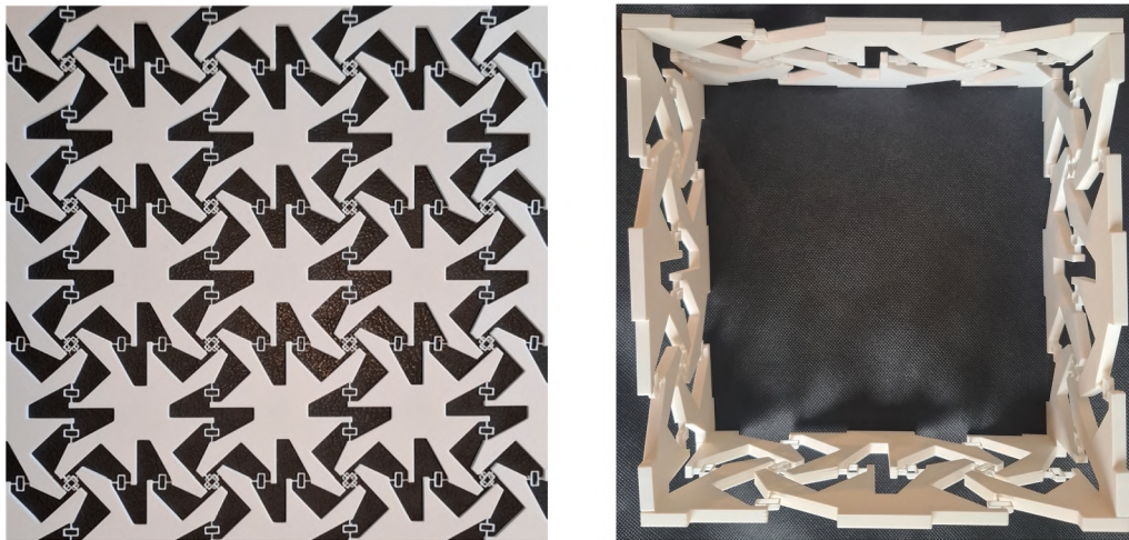
Fig. 2. The mockups printed as single plane layer and as a 3-D box, based on the concept of auxetic Heuristic Molecule.
