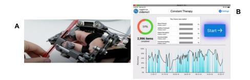
**Figure 1**: A. The Handexos system is a device with multiple actuators for each finger that allows for finer motor control. B. Screenshot from the Constant Therapy App.
