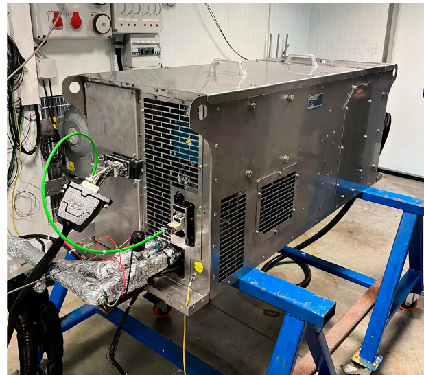
Figure 12. Experimental setup of BTMS experimental validation done in Microelettrica Scientifica cooling system division.
