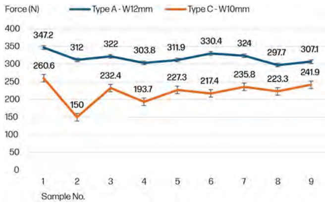
Figure 9: The results of destructive testing of the connections in Newtons.
