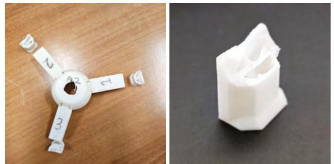
Figure 12: An image of the sample after testing showing the full connection (left) and the failure points at the fingers (right).
