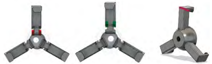
Figure 11: The potential failure points of the connection.
