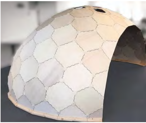
Figure 1: The ECHO Shell: A segmented lightweight shell structure.
