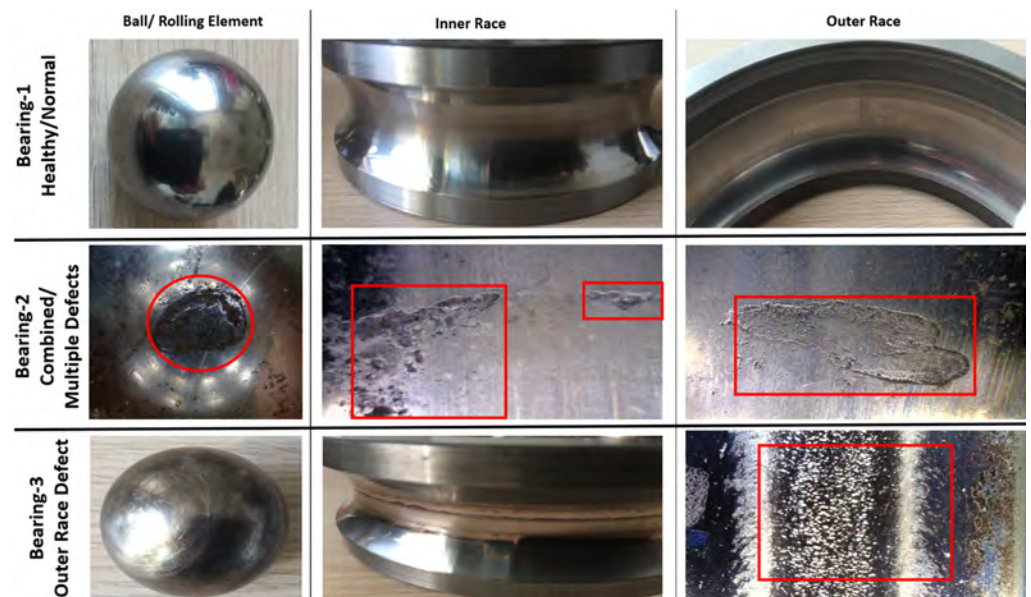
Figure 7. Healthy and defected bearings considered in case study-1.
