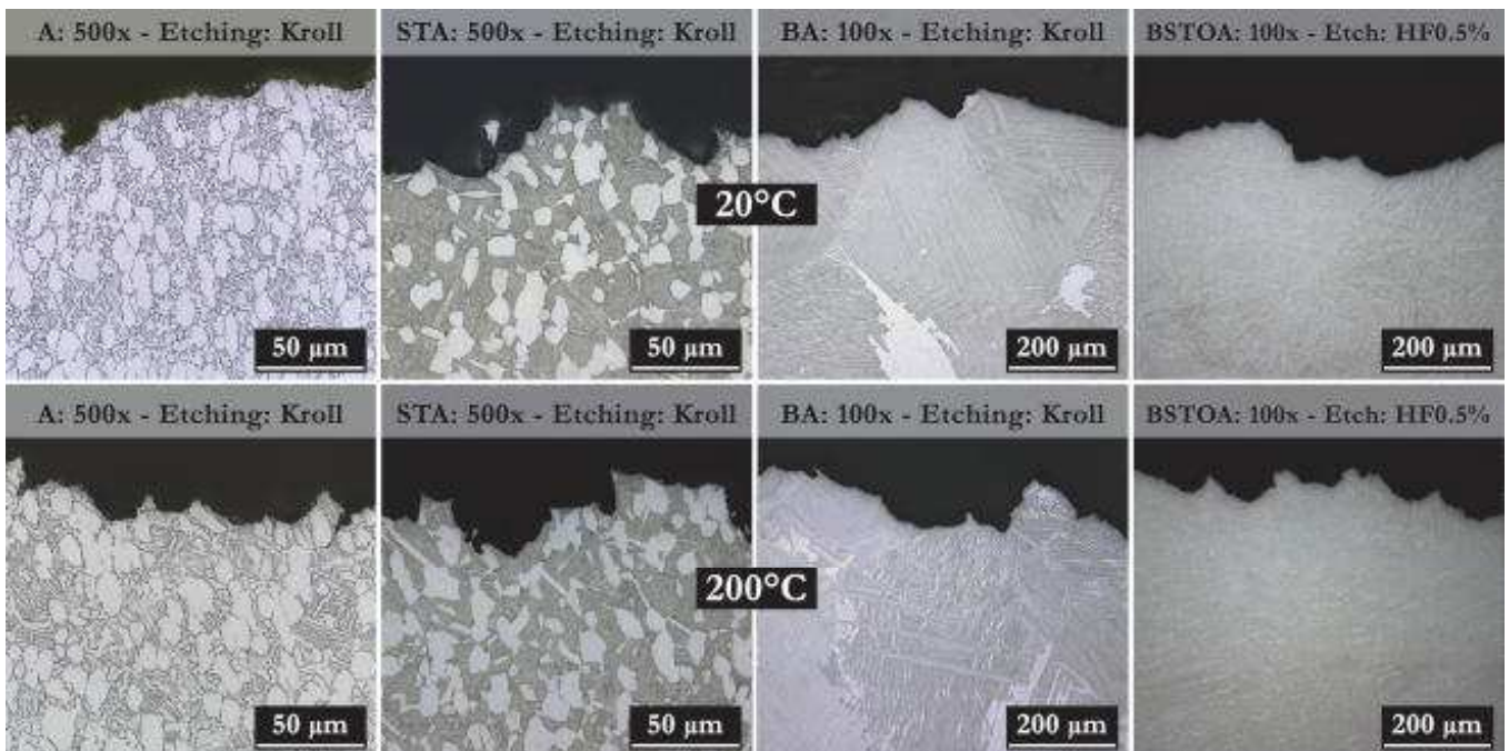
Figure 12: Longitudinal cross-section of fracture surface of impact test specimens examined at 2 mm distance from the notch. To highlight differences, fracture surface of the impact toughness performed are compared at +20 °C and +200 °C.
