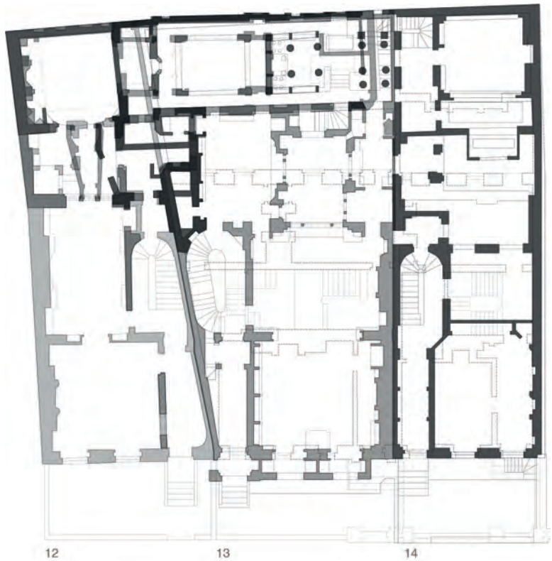
John Soane house-museum in Lincoln's Inn Fields, London, 1792-1833. Redrawing by the author (2022) of the main transformation phases of the house. In light grey are depicted the initial change of the first house unit (12); in medium grey the changes occurred with the first expansion (13) from 1807 to 1821, and the new entrance of the house; in dark grey the latest ones in 1833 involving the entire property (12,13,14).
