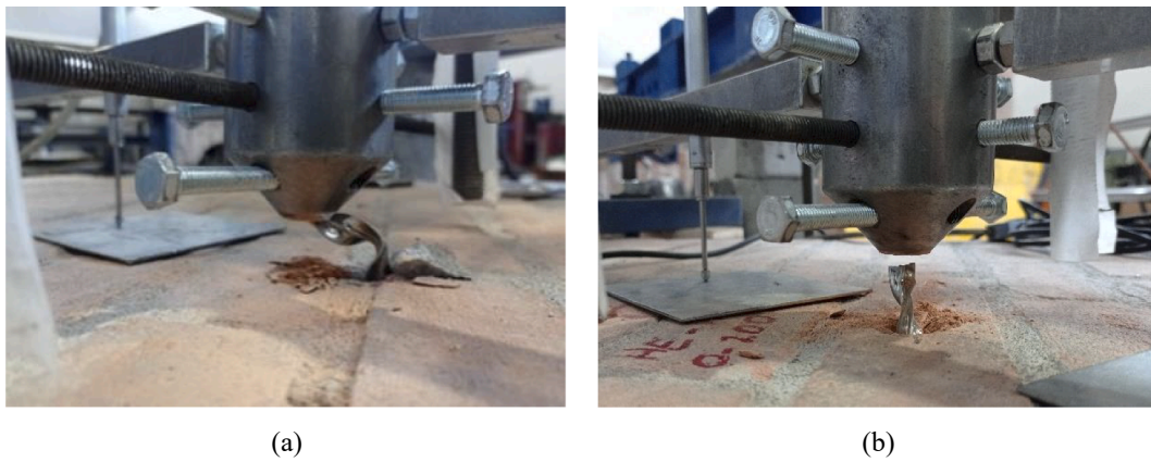
Fig. 12. Twisted bar in compression (a) and failure in tension (b).
