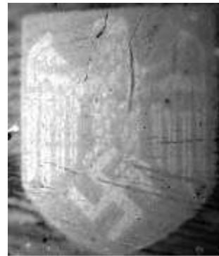
Fig. 13 Camo paint transparent in the 3-5 \mu\text{m} waveband.
