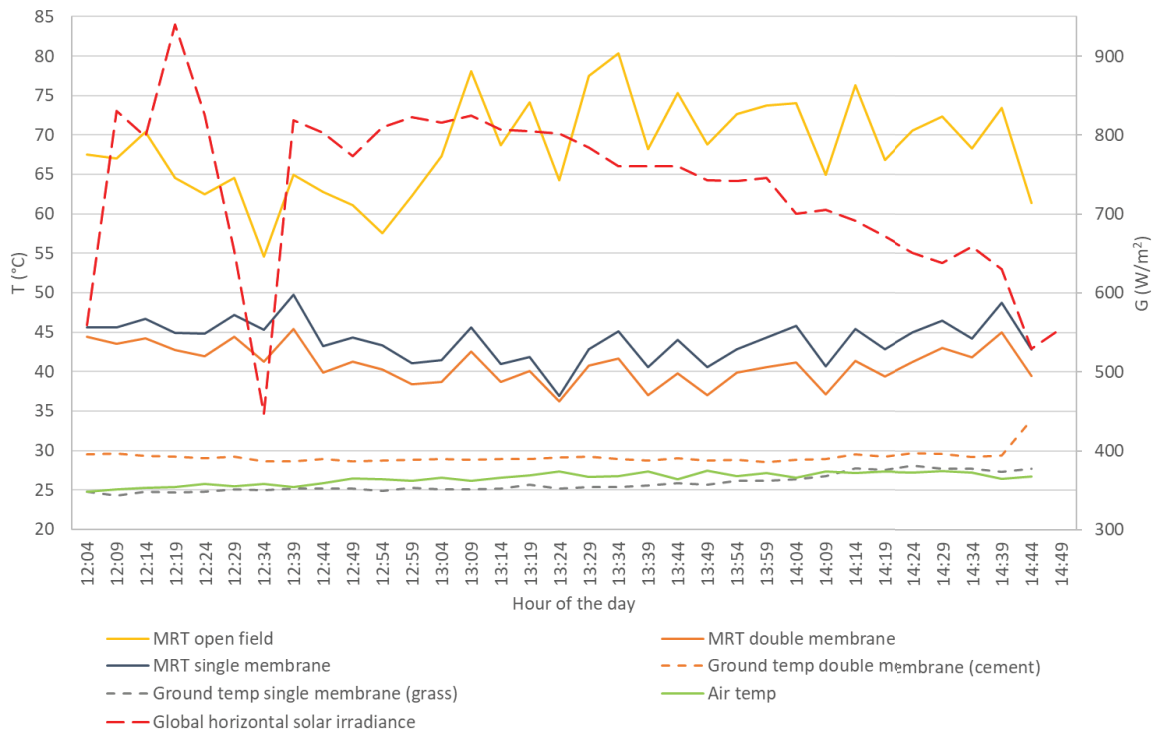
Figure 4: Monitoring data in a representative day of the first part of the campaign (“day 1”)
