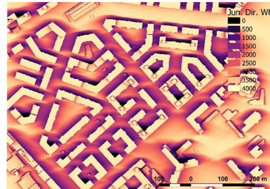
Figure 8: Direct solar irradiation representative of an average day in June (Wh/m 2 *day).
