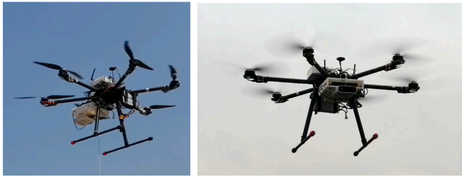
Fig. 11. Vision equipment mounted on drone.
