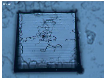
Figure 4 - Microlens cracked after the oven treatment
