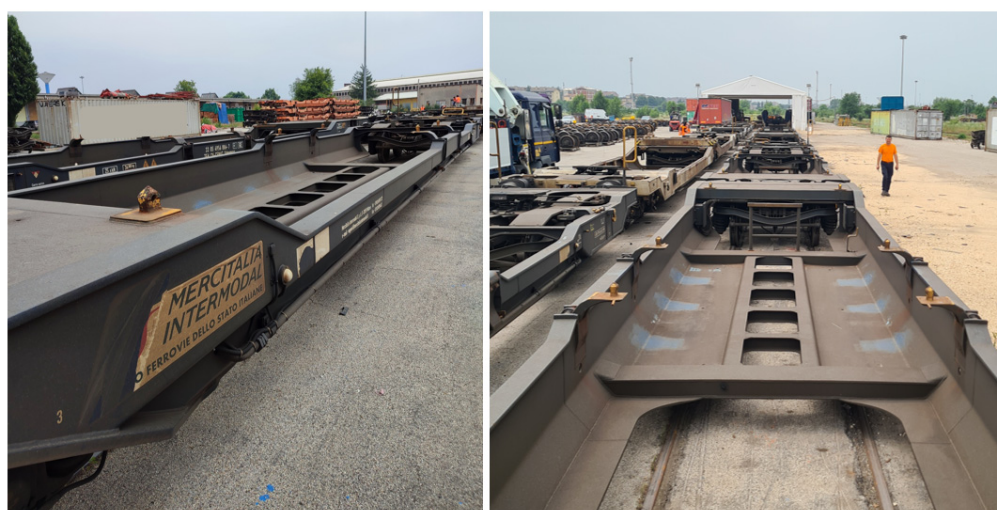
Figure 1. T3000 articulated freight wagon (on field views).
