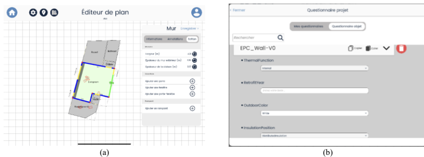
Figure 10 – Italian case study, geometrical model enrichment, (a) information automatically collected through the scanning of a wall, (b) wall's questionnaire. Authors' elaboration.
