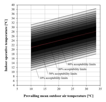
Figure 3 Acceptable operative temperature ranges for occupant-controlled naturally conditioned spaces
