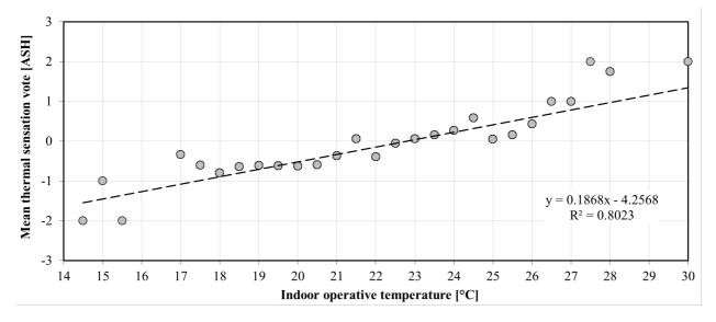
Figure 1 Example of a correlation between the mean thermal sensation vote (ASH) and the indoor operative temperature for one building of the ASHRAE RP-884 database: Oxford UK (summer), NV building #1
