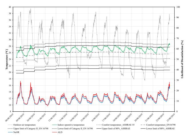
Figure 7 Indoor operative temperature distribution, comfort temperature thresholds (left scale), according to EN 16798 (PPD < 10%) and ASHRAE 55 (80% acceptability limit) and the predicted percentage of dissatisfied (right scale) obtained applying the NaOR and ALD indexes, respectively.
