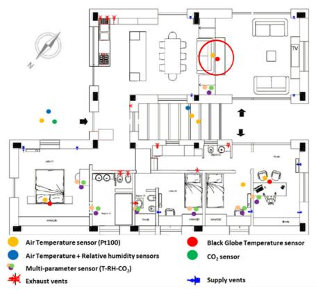
Figure 6 Plan of the building and sensors' location. The sensors selected for the analysis are circled in red
