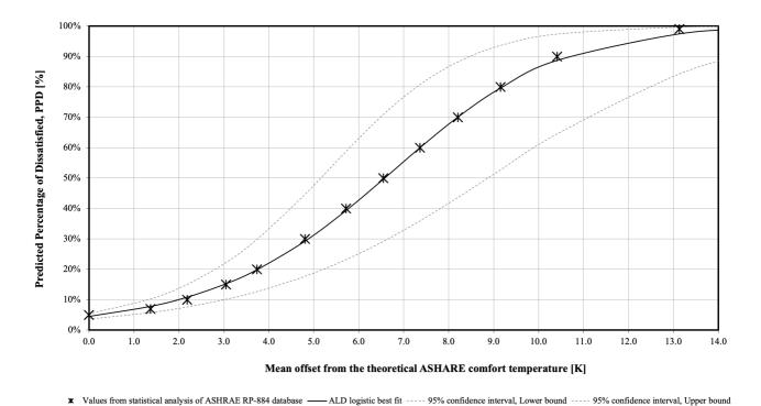
Figure 2 Predicted Percentage of Dissatisfied (PPD) versus the mean offset from comfort temperature obtained by the elaboration of data from ASHRAE RP-884 database. The interpolating logistic curve is the proposed ASHRAE Likelihood
