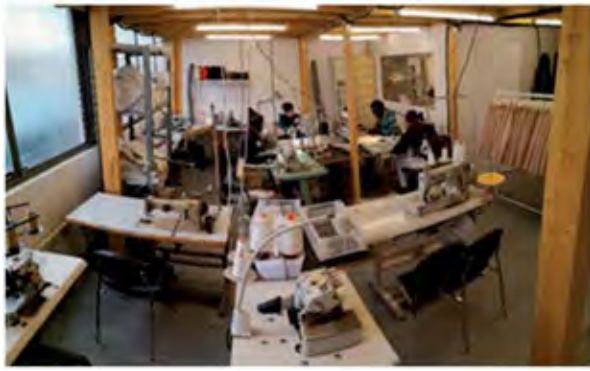
Figure 4. The group production island layout tested at Coco&Rico production facilities.
