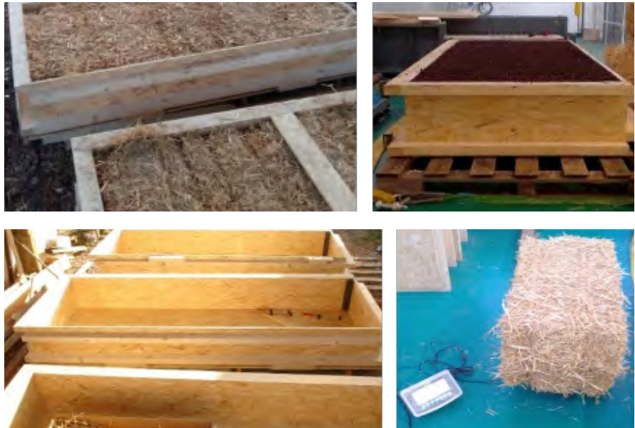
Figure 6. Panel structure, straw bale, and panel structure filling: straw and cork: Photos by Reaes Pinto.
