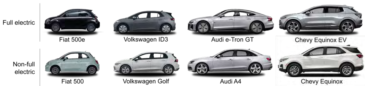
Figure 2 Visual comparison between fully and non-full electric models, illustrating the aerodynamic-driven design prevalent in e-cars.
