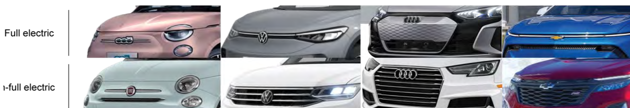
Figure 3 Comparison of front grill design in four different brands depending on the propulsion system.
