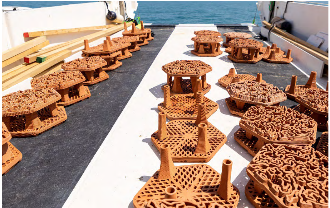
Fig.8 Fig.9 3D printed tiles, designer: Archireef, University of Hong Kong (Christian J. Lange, Lidia Ratoi, Dominic Co Lim, Jason Hu from Robotic Fabrication Lab, Vriko Yu, David Baker, Phil Thompson from Swire Institute of Marine Science - SWIMS), in partnership with Chinese Agriculture, Fisheries and Conservation Department (AFCD), San Kung Peninsula, Hong Kong, 2020. Photo courtesy Archireef and Hong Kong University.
