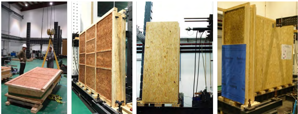
Figure 7. Elevating the panel and assembling the panel on the base element: Photos by Reaes Pinto.
