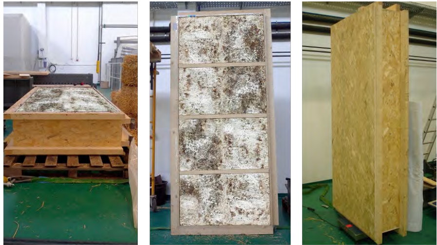
Figure 18. Prefabricated exterior wall module with fungal mycelium insulation: Photos by Reaes Pinto
