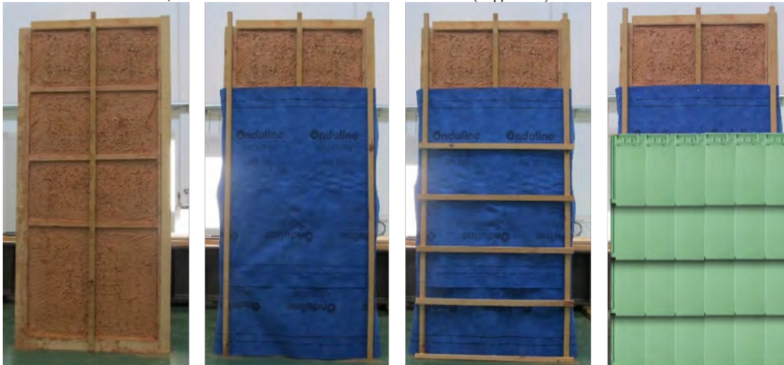
Figure 8. Exterior finishing assembly test with flat ceramic tile: Photos by Reaes Pinto.
