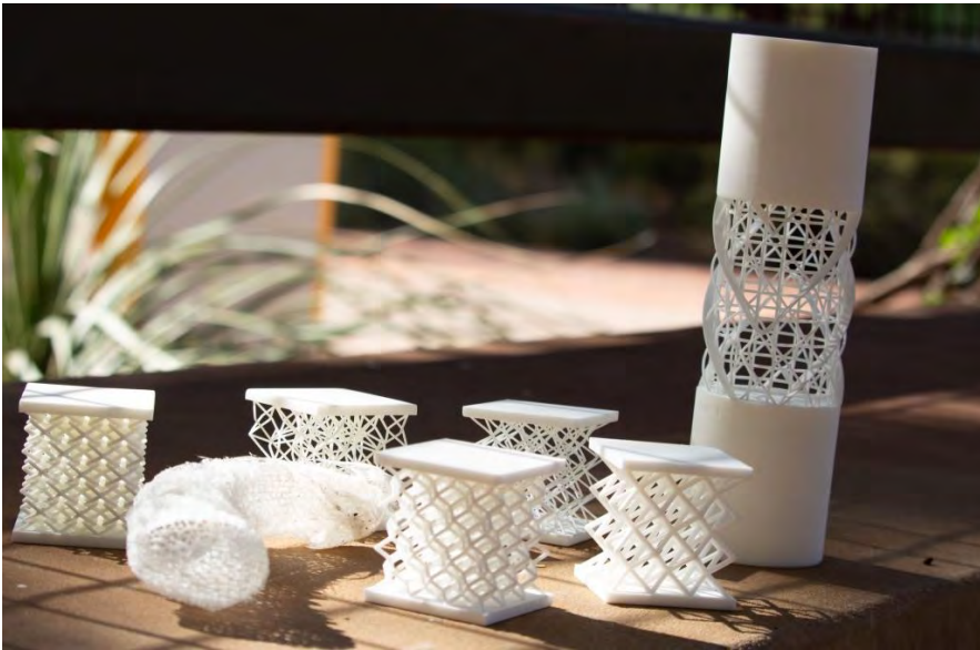
Fig.4 Optimized structure inspired by butterfly wing scales to maximize stiffness and density (Pelanconi et al., 2019).
