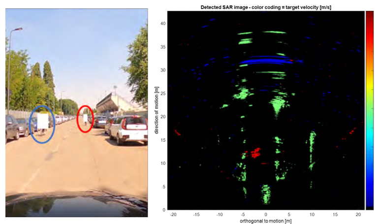
Figure 14. SAR imaging of moving target in an open road (forward-looking configuration): (left) camera image of the acquired scenario (right) RGB color-coded SAR image with the static scene (in green) and the detected moving targets (red and blue). In the red circle in the camera image, a cyclist moving in the direction of the ego-vehicle. In the blue circle, a cyclist moving in the opposite direction.
