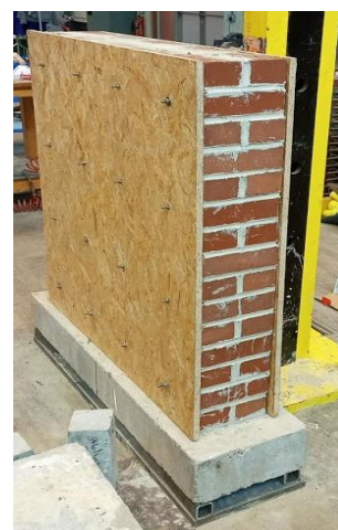
2-sided retrofitted wall
