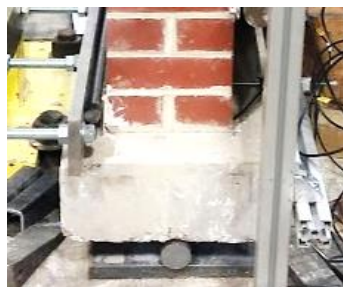
d) Roller under wall specimen
