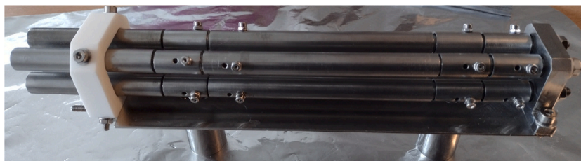
Fig. 4. Photograph of the ion trap used in the experiment, before it was installed in the vacuum chamber and wired for the voltage supplies. The electrodes are made of molybdenum, and the support frame is mostly made of stainless steel. The white supporting element is made of macor.
