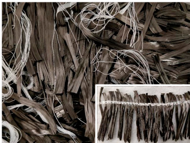
Figure 2. Carbon fibre waste produced from the stitching process.
