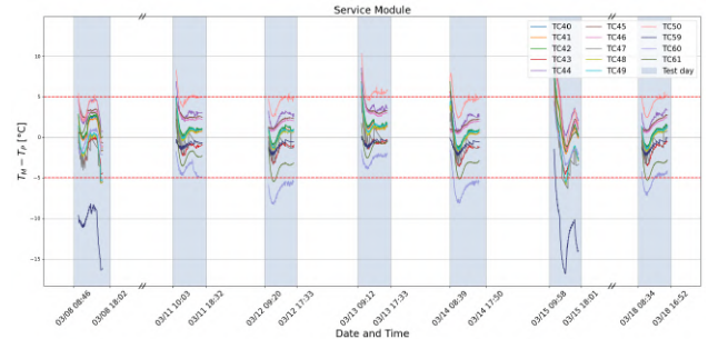
Fig. 11: Deviation from test results for the TCs of the service module.
