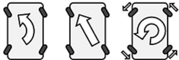
Fig. 4 Diagrams of the Rover's different movement modes
