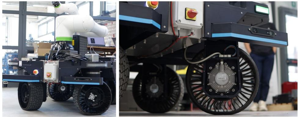
versatile and cooperating robotic platform for the creation of brick structures.
