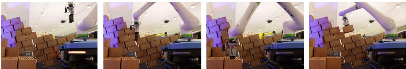
Fig. 12 Operation sequences of BRIX constructing a wall in Bari at SAIE fair 2023
