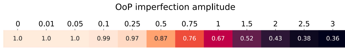
Fig. 6. Heatmap with the knockdown factors based on linear buckling analyses.
