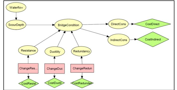
Figure 4 BPN tool for the bridge.
