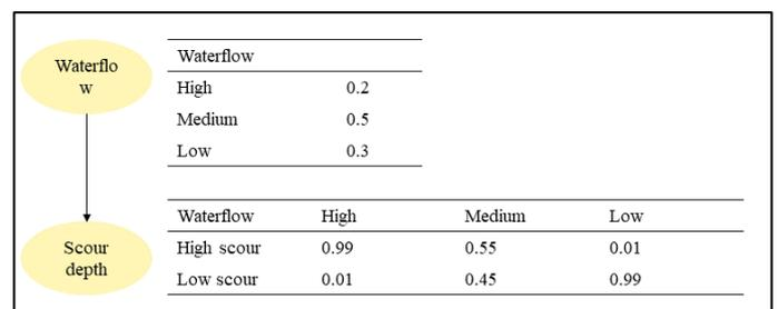
Figure 6 Probabilities assigned to the water flow and the scour nodes.
