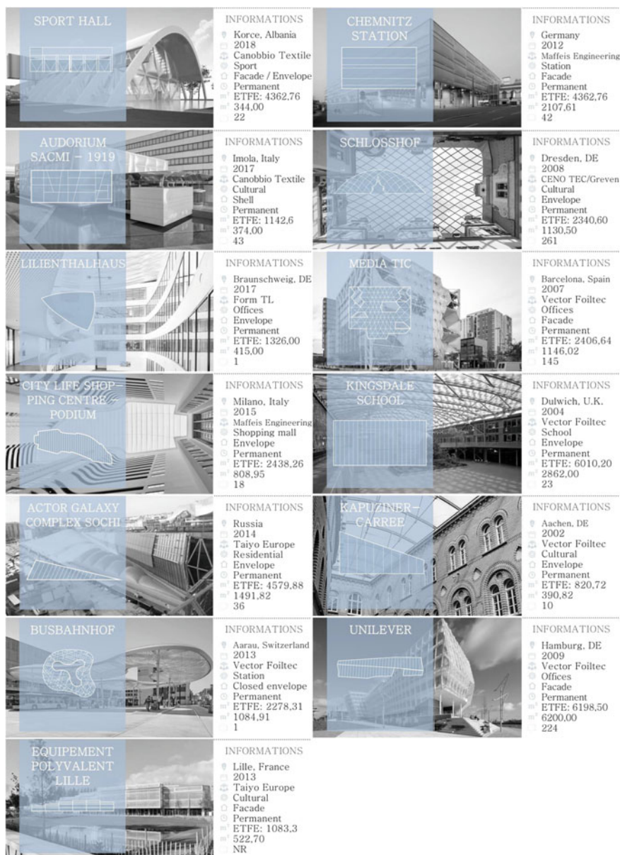
Fig. 1 Building textile envelope solutions and their dimensions as case studies for applying two eco-efficiency principles. Reproduced from (Monticelli and Zanelli 2020)
