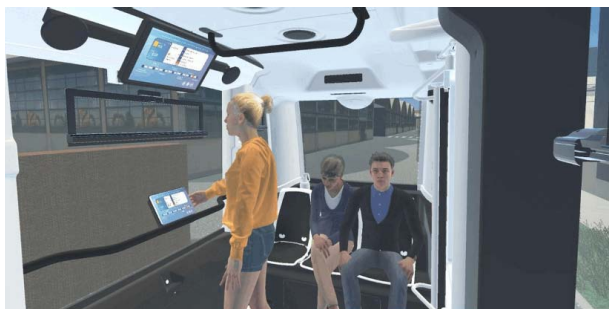
Figure 2: A representation of the Unity 3D interaction scene was created for testing inside the vehicle. There are two interactive displays in the scene, one above the user's head and the other on the armrest rail.
