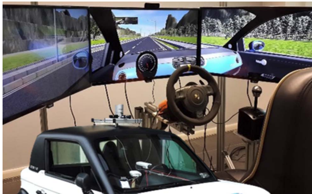
Figure 1: Driving Simulator Setup for the test dataset [7].
