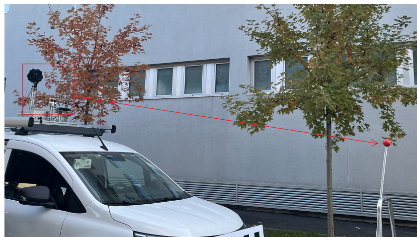
Figure 15. Validation setup: the sensor system is shown on the left, while the red spherical target is shown on the right, with its center selected for computing the azimuth and elevation error deltas.
