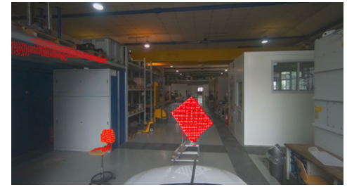
(b) Point cloud (Red dots in the image) transformed into the camera frame using the pose estimated through the proposed Hybrid GA-PSO optimization.
