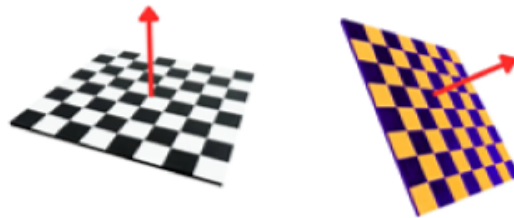
Figure 4. Illustration of the angular error between the checkerboard normal vectors. The black and white checkerboard represents the plane observed in the camera frame, while the orange checkerboard corresponds to the same plane represented in the LiDAR frame. The red arrows denote the respective normal vectors in each coordinate frame, and the angular discrepancy between them defines the alignment (normal-to-normal) error.
