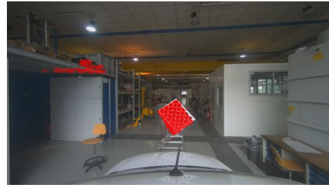
(a) Point cloud (Red dots in the image) transformed into the camera frame using the pose estimated through the Gradient Descent optimization.
