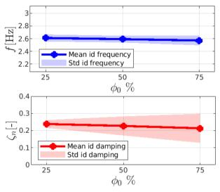
Mean and standard deviation of the identified frequency and damping at different longitudinal cyclic lever position. Input longitudinal acceleration. Output: longitudinal cyclic rotation. Mean and standard deviation of the identified frequency and damping at different lateral cyclic lever position. Input: lateral acceleration. Output: lateral cyclic rotation.
