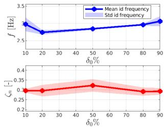
Mean and standard deviation of the identified frequency and damping at different collective lever position using heavy, long collective. (3.03 kg, 800 mm) Input: vertical acceleration  $\ddot{Z}$ . Output: collective rotation  $\delta$ .
