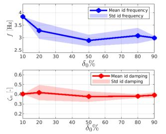
Mean and standard deviation of the identified frequency and damping at different collective lever position using light short collective (1.21 kg, 350 mm) stick. Input: vertical acceleration  $\ddot{Z}$ . Output: collective rotation  $\delta$ .
