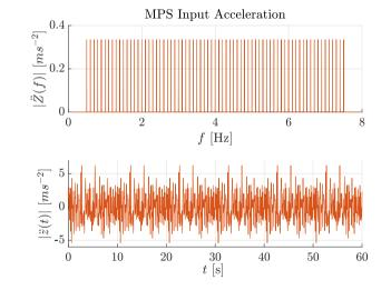
The pilot-vehicle system is excited by a pseudo-random waveform in the frequency band [1, 7.5] hertz with limited RMS acceleration level:
