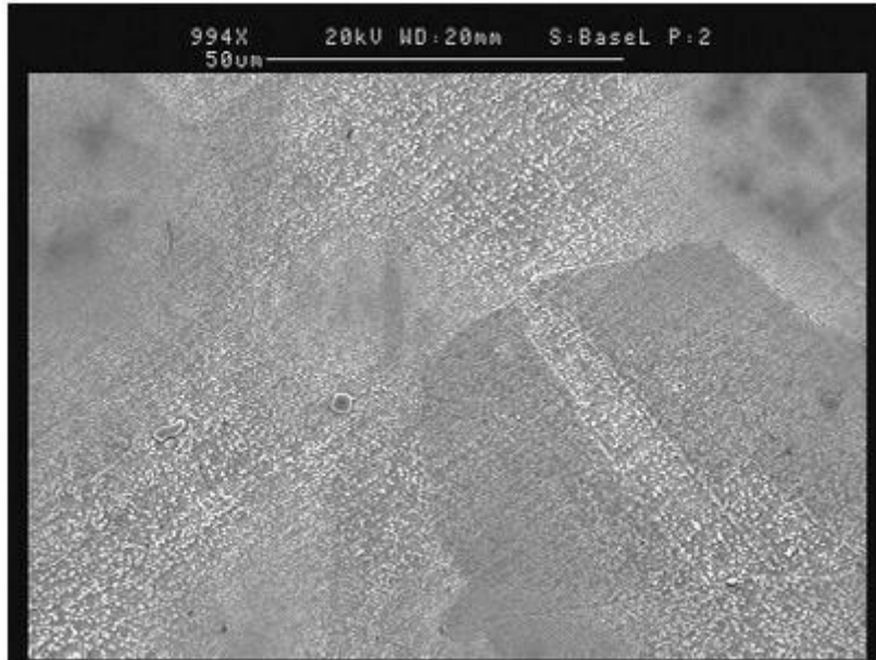
Figure 1 Microstructure of Inconel 718 in the initial state, SEM image.
