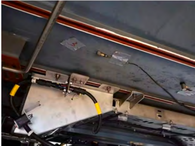
Fig. 7. In-situ tests for the carbody vibration.
